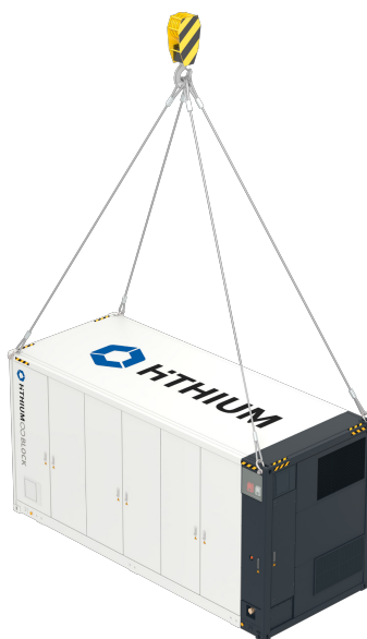
Fig 4-2 Lifted via Crane
