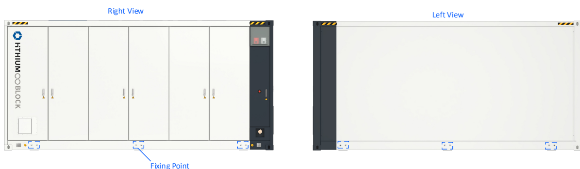
Fig 5-1 Fixing Points of the ESS Container
