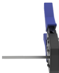
Fig 5-34 Crimp the Network Cable (for Reference only)
