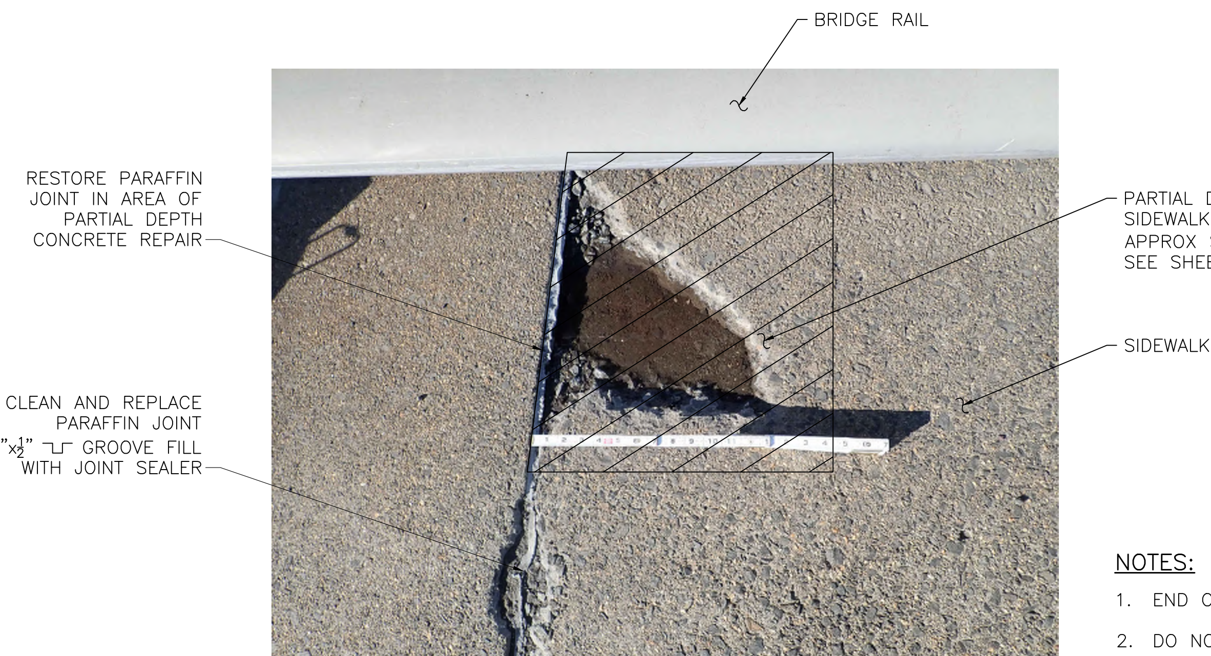
PARTIAL DEPTH CONCRETE SIDEWALK REPAIR
