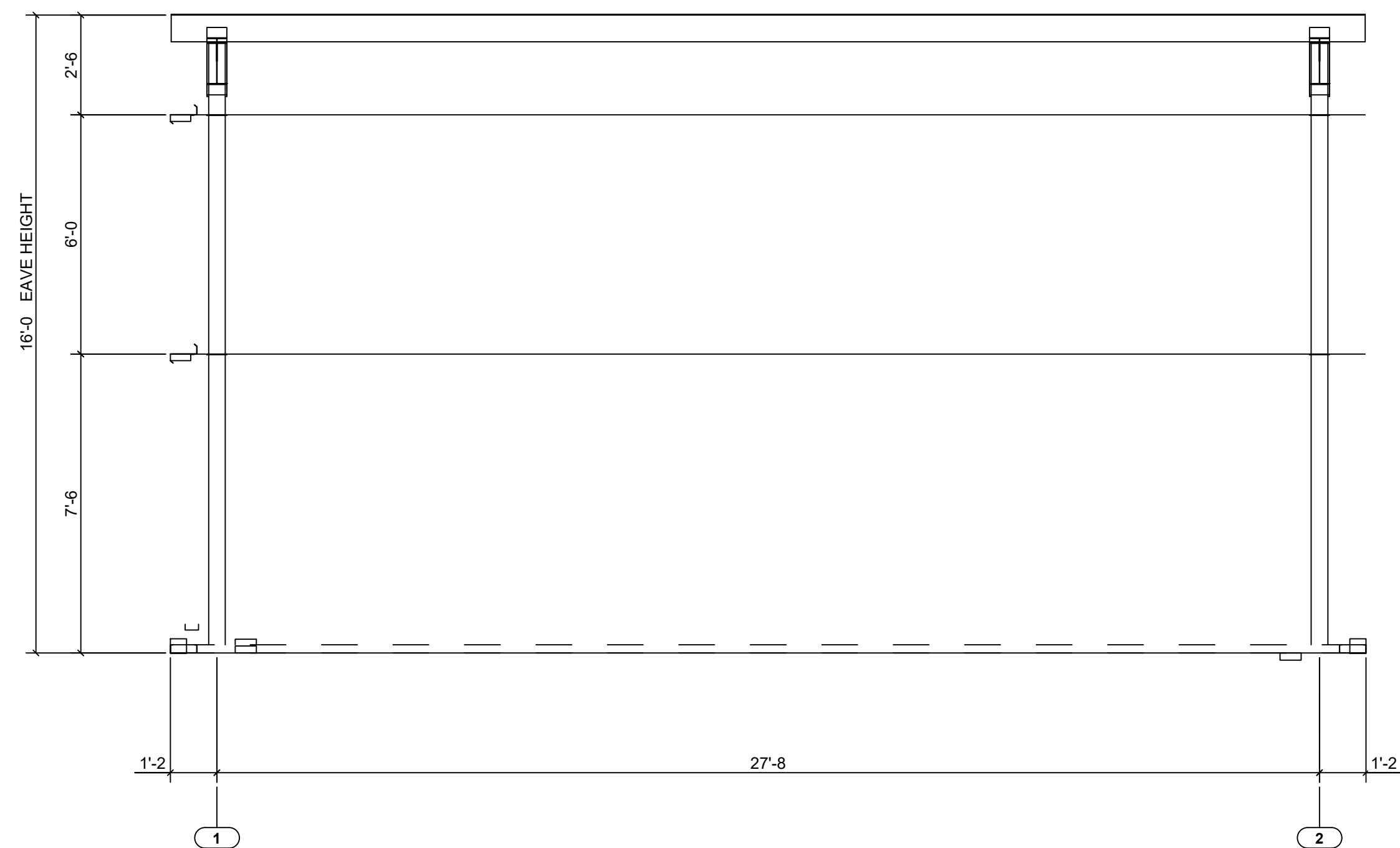
Sidewall Framing SWA at Grid Line A
